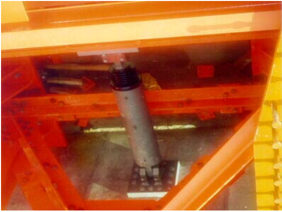
Fig. 22: Sample for anchoring of device to concrete and steel structure
